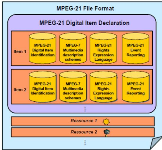
Figure 4. Hierarchical metadata structure within a MPEG-21 file [18].
