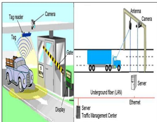
Figure 3: E-ZPass System (on the left – blocked road line, on the right – open road line)
