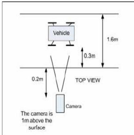
Figure 1 Camera set up for the wheel detection system
